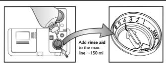
The rinse aid dosage can be adjusted to the detergent used. The lower the setting, the less rinse aid is dispensed (factory setting: position 4). Press the button to open the cover B. Using a coin or similar object, turn the arrow to the desired setting. After adjusting the rinse aid setting, shut the cover again.
